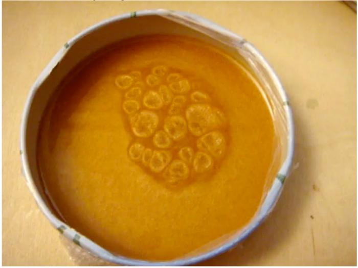
Gold paint dissolved in acetone. Put it in a shallow dish. Cover it so that the acetone does not evaporate. Let stabilise and then remove the cover. Evaporation of the acetone causes the top layer to cool thus starting convection.
