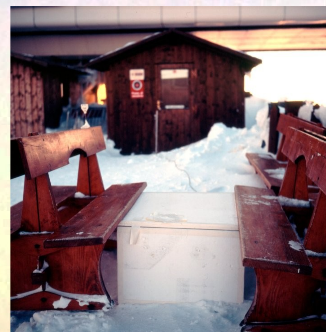
REFIR-PAD installed at Monte Gomito in a polystyrene thermal shielding enclosure
