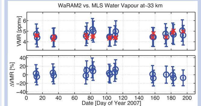
Figure 4: (Upper panel) H<sub>2</sub>O VMR from WaRAM2, indicated by blue circles, with error bars, at ~33 km, compared to MLS data, indicated by red crosses (see text). (Lower panel) Same data as above, but given in relative units with respect to MLS.
