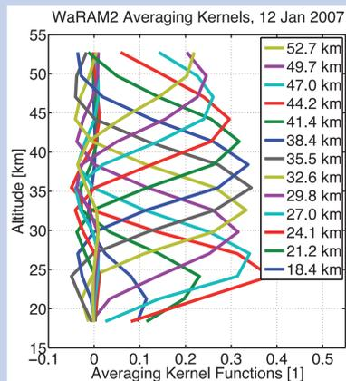
Figure 1: Selected averaging kernels (AVK) of the WaRAM2 retrieval on 12 Jan 2007. The legend indicates centre altitudes of the individual retrieval grid layers. Altitude resolution ranges from 8 to 12 km.
