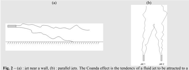
Fig. 2 - (a): jet near a wall, (b): parallel jets. The Coanda effect is the tendency of a fluid jet to be attracted to nearby surface.
